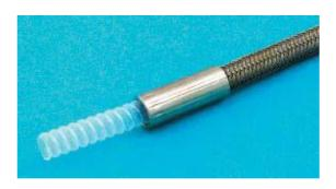
We recommend PTFE when you want a high durability and the application demands high chemical resistance. The hose is designed with an corrugated inner tube from PTFE and an outer braid in stainless steel (for standard AISI 304) is used. We also produce high performance hoses with innertubes in other fluoroplastic materials such as PFA, ETFE and PVDF or with a covering from Hytrel®.
