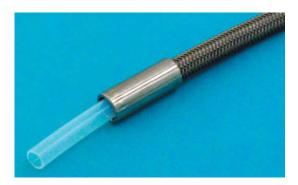
We recommend PTFE when you want a high durability and the application demands high chemical resistance. The hose is designed with an straight inner tube from PTFE and an outer braid in stainless steel (for standard AISI 304 is used - 316L available upon request). We also produce high performance hoses with innertubes in other fluoroplastic materials such as PFA and ETFE or with a covering from Hytrel<sup>®</sup>.
